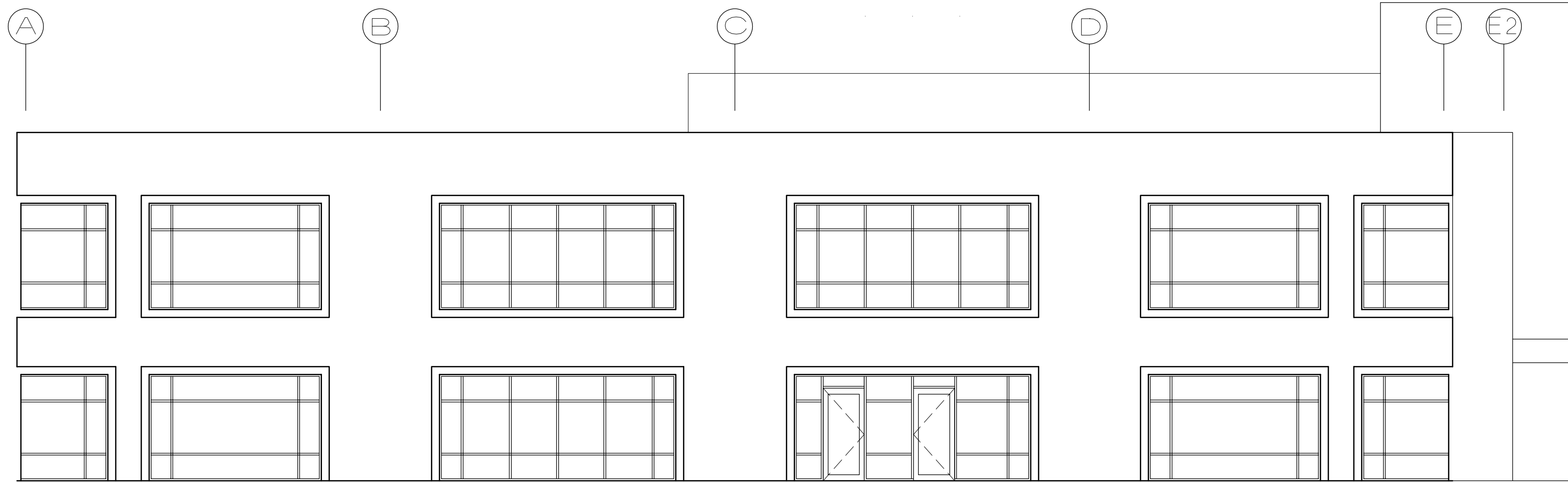
4 WEST EXTERIOR ELEVATION 1/8" = 1'-0" 1/8" = 1'-0" 0 2' 6' 12' 24'
