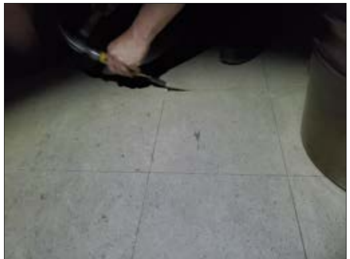
24. Samples 18A-18C: 12"x12" beige VFT with black specks and yellow mastic, first floor
